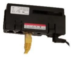
2. Insert the communications module into the top of the device with the tabs facing outward. The module will click into place when it is fully inserted.
