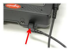
2. Connect the HDMI end of the communication cable to the back of the device.
