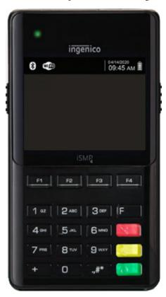
**Caution**: If the Ingenico iSMP4 is plugged into the charger, and the charger is plugged into an outlet, do not power the device on or off. Unplug the device first, and then power it on or off. Failure to do so can result in damage to the device. For more details, refer to the iSMP4 documentation.
